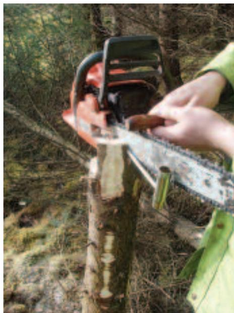
Now the chainsaw can be sharpened while the operator is standing up.
