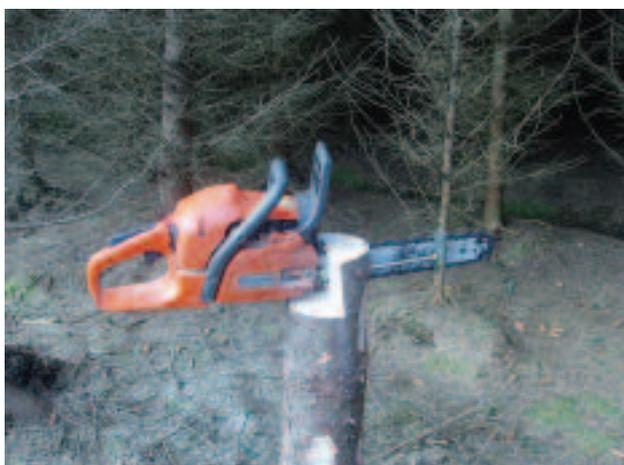
**Step 6:** Insert the chainsaw with the blade in the opening and with the machine resting on the step (if the spikes on the chainsaw have been maintained, ram them into the upright) and fix the machine in place with the nut tightening key.
